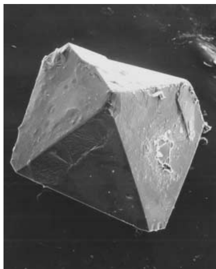
Figure 1. SEM image of a cyclohexamantane crystal magnified 150 \times .
